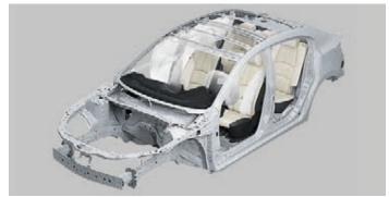
Advanced dual front air bags\* that utilize inflators with both crash zone and passenger's seat weight sensors are standard on all Mazda models - as are dual front side impact air curtains with coverage for front and rear passengers.
